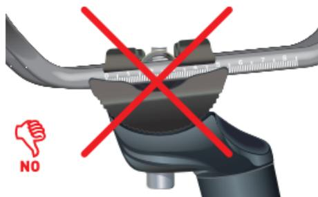
7. the jaws should not cause deformation or damage to the saddle frame
